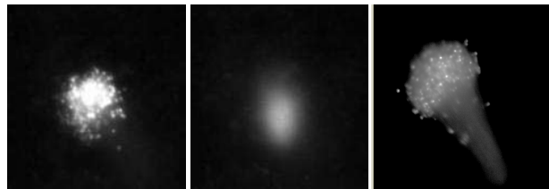
figure 4.a. The contact surface of the IR-brush on the canvas (left). 4.b. IR-light on the canvas when the brush is near the canvas (middle). 4.c. The contact surface when the IR-brush is pressed on the canvas (right).
