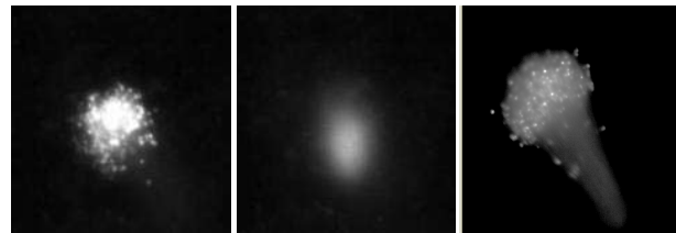
figure 4.a. The contact surface of the IR-brush on the canvas (left). 4.b. IR-light on the canvas when the brush is near the canvas (middle). 4.c. The contact surface when the IR-brush pressed on the canvas (right).
