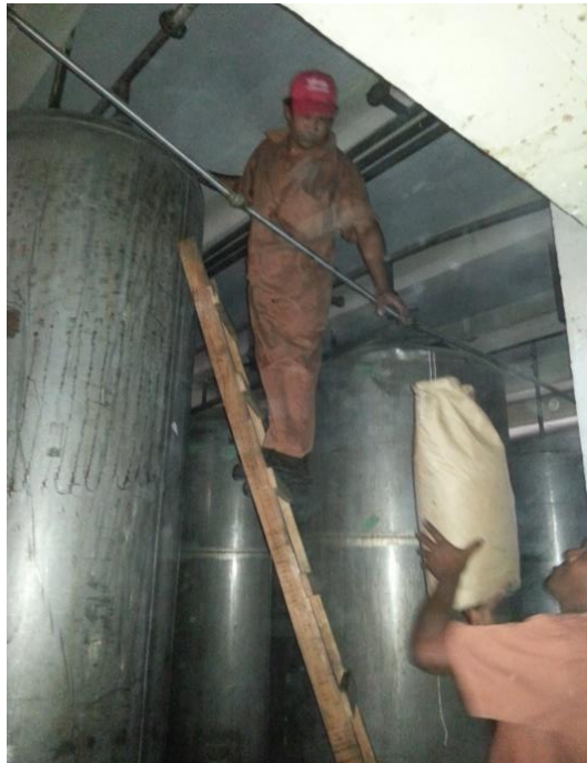
Fig.S4: Preparing the industrial rum filter with regenerated GAC.
