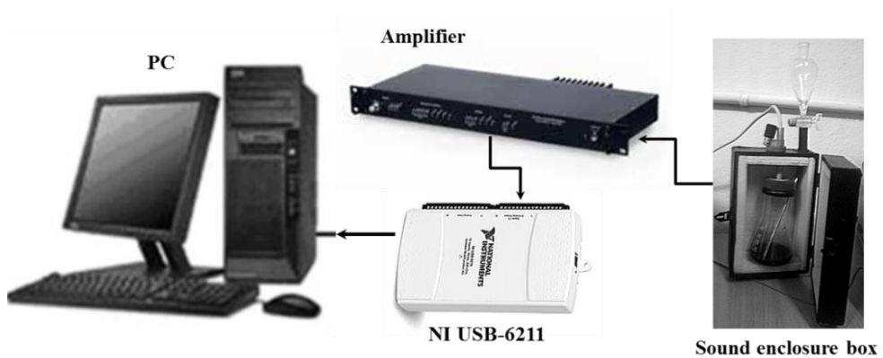
Fig.2.5: Scheme of the experimental set-up for signal capture and processing
