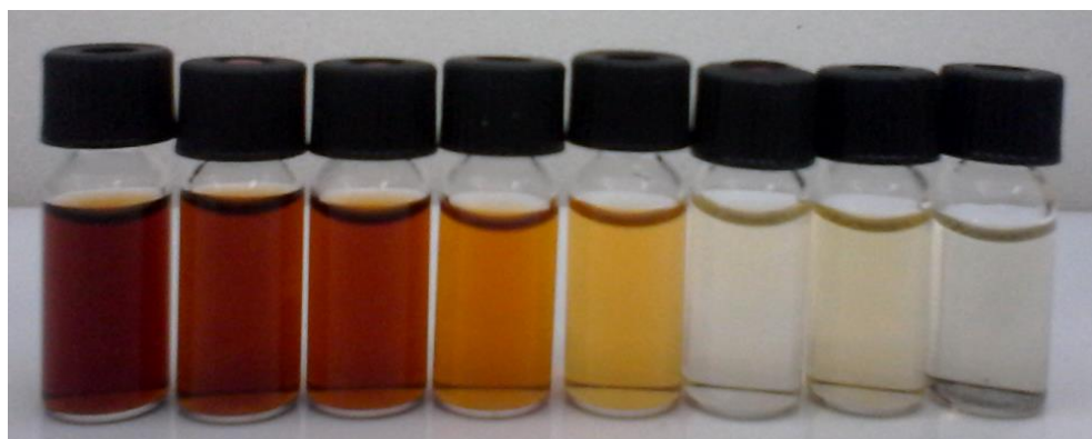
Fig. 3.13: Color profile of extracted solutions of the different GAC samples in the rum filter. The color intensity is decreasing from the top (left) to the rum filter's bottom (right).
